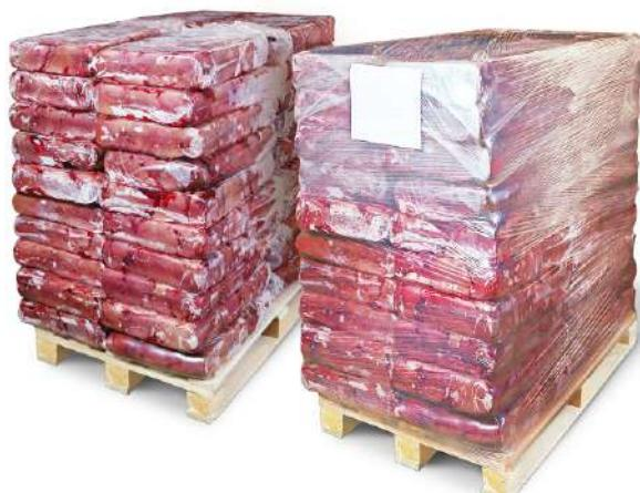
Products packed in bags or boxes are stacked on a euro-pallet with dimensions of 800\*1200 mm, according to the scheme in the photo. The pallet is tightly wrapped with a stretch film of at least 7 layers; the stretch film is attached to the pallet legs. Pallet sheets with information about the product are placed in the upper third of the pallet, on the narrow and the wide sides.
